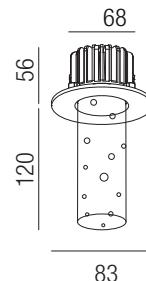
**Bubbles**, IP20, 8W, 710lm, 3000K LED
